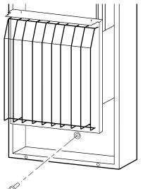
Figure 11 - Installing Bottom Mounting Screw
